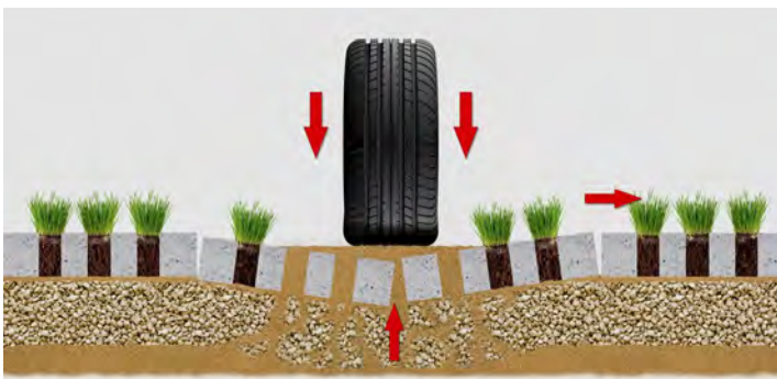
Fig. 7 Pre-cast concrete grass pavers under load
